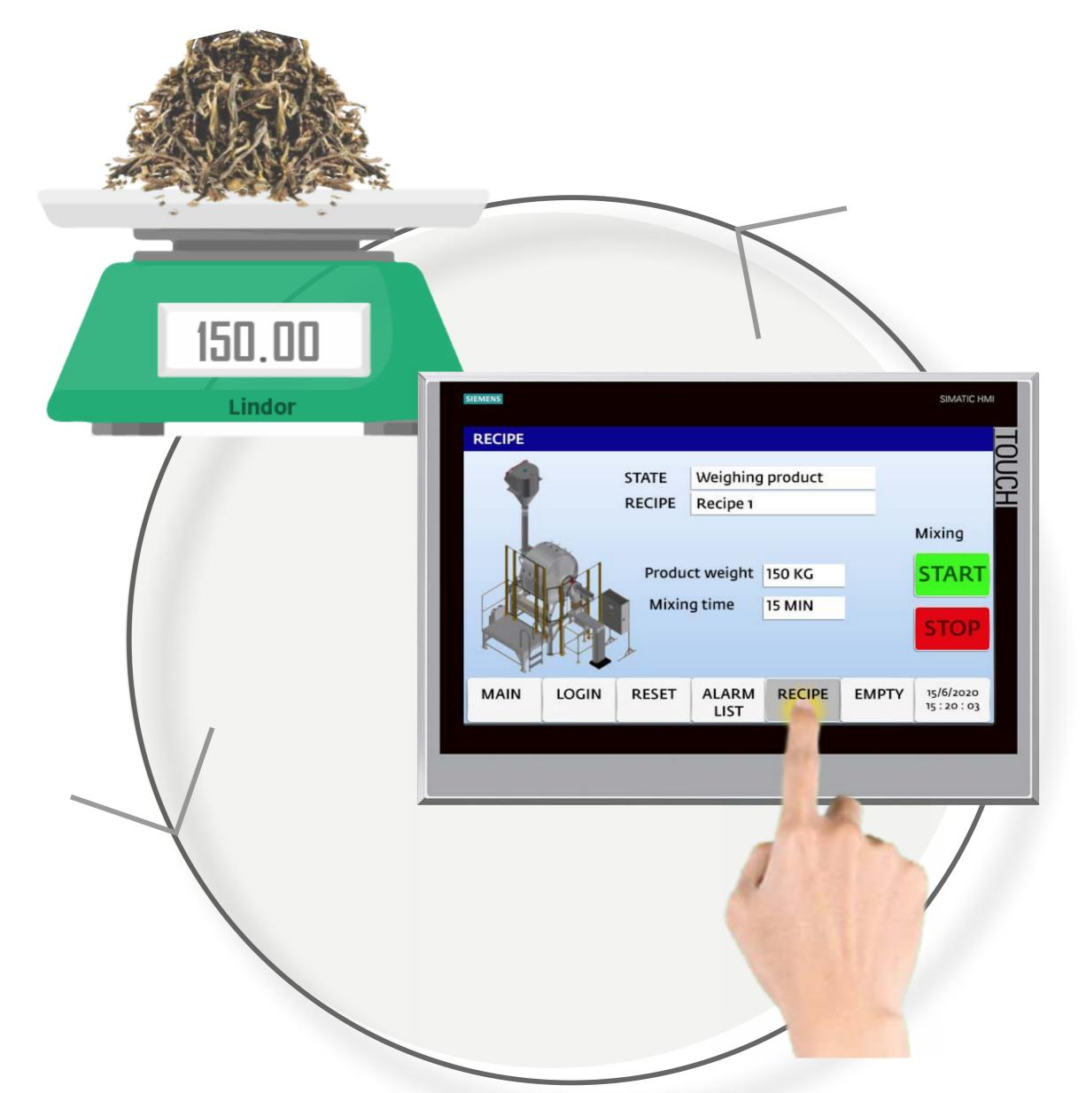
Thanks to the installation of load cells in the hopper, the operator ensures that only the correct amount of product ingredients are fed into the mixing drum at any given time.
